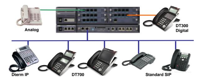
A standard SIP terminal uses two channels.
