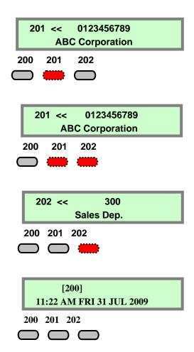
R3 Version License is required for Caller ID Sub-line. NEC terminals that support Caller ID Sub-line are DT300/700, Dterm 80/85 (series i Digital), Dterm 85 IP (series i IP), Dterm 70/75, (series E Digital) Dterm 75 IP (series E IP), SP30, and MH240.
