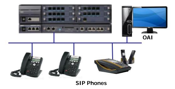
Property Management System (PMS), Station Message Detail Recording (SMDR) and Message Waiting (MW) is supported on the standard SIP terminals. (PMS system license is required.)
