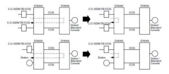
A trunk call (C.O./ISDN/TIE/CCIS) over CCIS is transferred or forwarded to the VRS for Delay Announcement- UCD within the same office as the original incoming trunk.
