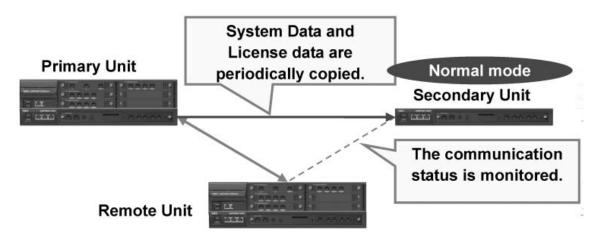
**Failover Mode Operation:** If a communication failure occurs between the Main Site and Remote Site, Remote Unit automatically resets itself, and sends a connection request to the Secondary Unit. Then Secondary Unit goes to Failover Mode and starts controlling call processing of Remote Unit. In Failover Mode, the system data and license data copied during Normal Mode will be effective.
